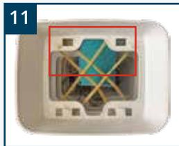
**11** Position the PM2.5 sensor so that it fits snugly into the space along the long edge of the shield, between the final two plates.
